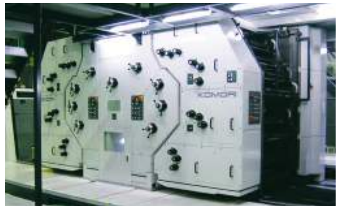
証券用オフセット印刷機 (CURRENCY LT-832IIA) An offset printing machine for printing securities (CURRENCY LT-832IIA)
