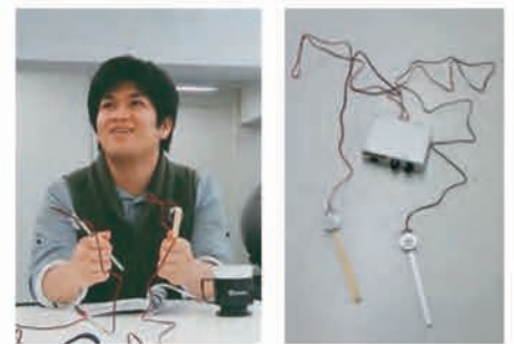
触音器(金属の棒と木材の棒) Sound-feeling device (metal bar and wood bar)
